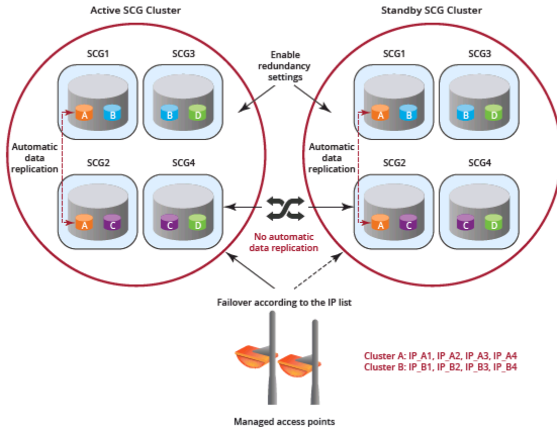
FIGURE 65 Cluster Redundancy for Active-Standby Mode
