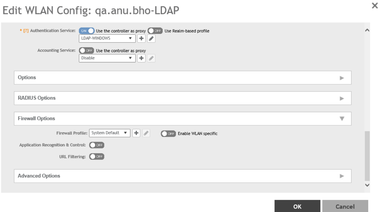
FIGURE 185 Apply the Application Control Policy to a WLAN
